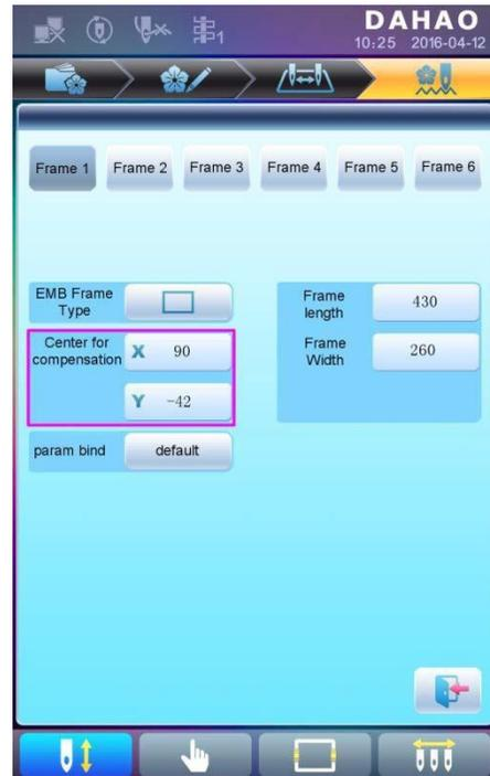
There are four parameters: "X direction center" means the distance at X direction between the frame center and X- direction position limitation optical coupler; "Y direction center" means the distance at Y direction between the frame center and Y+ direction position limitation optical coupler. "X direction frame size" means the embroidery range of the frame at X direction; "Y direction frame size" means the embroidery range of the frame at Y direction.
