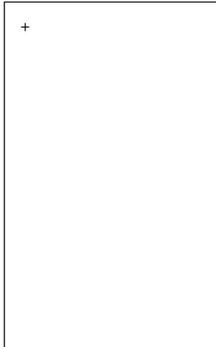
During the process of correction, a lot of crosses will appear on the screen. User should press the center of them. System receives the data of those points and saves them as standard data for correction.
