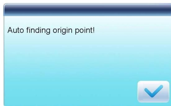
System will move the frame automatically and determine the origin according to the limit switch. So please ensure that the limit switch has been installed into the machine and activated.
